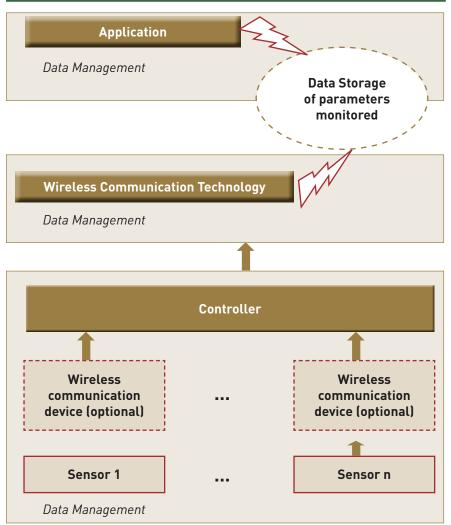
Fig. 2: Block Diagram of Water Quality Monitoring System based on Sensors [15]
