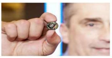
Intel's new device will include a Bluetooth low-energy radio, motion sensors, and components designed to rapidly and precisely differentiate between different types of physical activity. Krzanich said Curie will run "for extended periods of time" on a coin-size battery and would be available in the second half of the year.
