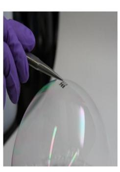
and that it is the in-line substrate manufacturing process that is the key innovation. Different materials could be used for the substrate and encapsulation layers, and different types of thin-film solar cell materials, including quantum dots or perovskites, could be substituted for the organic layers used in initial tests. But already, the team has achieved the thinnest and lightest complete solar
