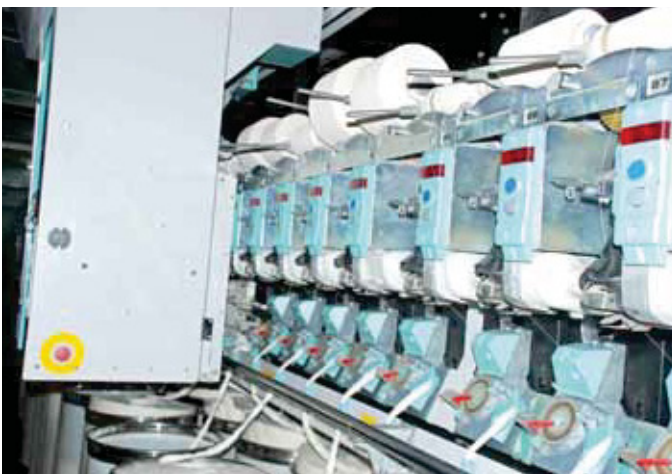
A view of fully Automatic Savio OE Spinning Machines with automatic piecing and cleaning facility installed at Rajapalayam Mills, Andhra Pradesh.
