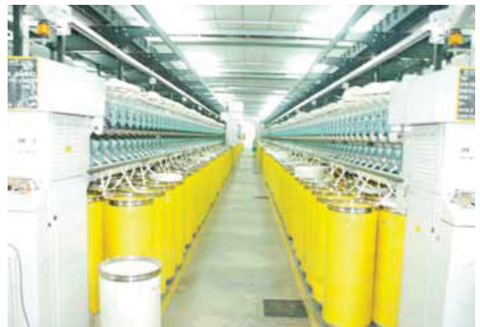
A view of fully Automatic Savio OE Spinning Machines with automatic piecing and cleaning facility installed at Rajapalayam Mills, Andhra Pradesh.
