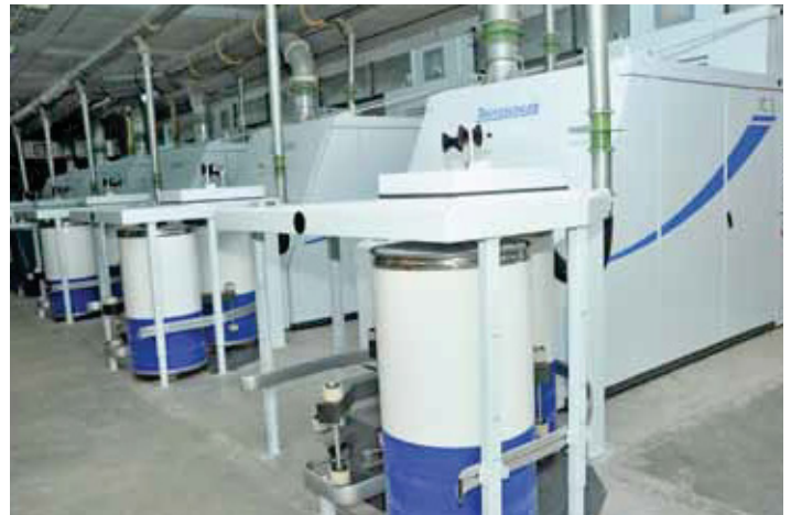
Newly installed Trutzschler Carding Machines at Rajapalayam Textiles (A Division of Rajapalayam Mills Ltd), Perumalpatti.
