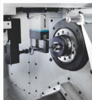
Our spindles known for their legendary precision (run out<0.003mm) are housed in a specially designed circular head stock without thermal distortion and expansion fitted with precision angular contact ball bearings and roller bearings that enable take up high axial and radial loads.
