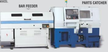
Our special accessories like bar feeder, bar puller, parts catcher, parts collection tray, high pressure coolant system etc. render the machine more versatile.
