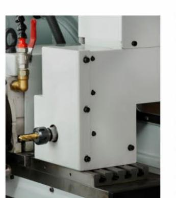
A customised Live Tool Unit driven by a servo motor which can accommodate one or two spindles based on component requirements for Axial Drilling/ Tapping or Milling operation (Max collet size ER 25 in case of single spindle and Er 20 in case of two spindles) is available optionally coupled with C Axis (Indexing Axis or continuous rotary Axis) which greatly improves productivity by reducing throughput time and also improves accuracies as component is finished in single set up.
